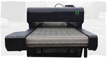
The new Adelco Pro-Cure Smart conveyor dryer range is available in four belt widths and five oven lengths, so you can customize your dryer to suit your individual curing requirements, for all digital and conventional textile ink systems. The Pro-Cure Smart is modular in design, making it the perfect option to add additional ovens to the dryer as your business grows.
