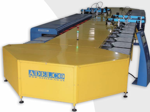
Bespoke oval design auto sock printer illustrated
