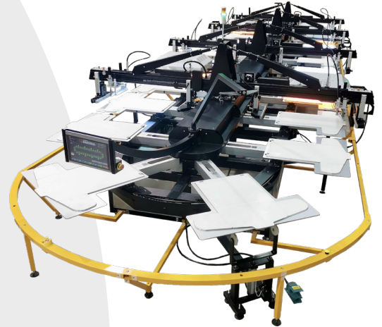
All Over Oval Printing Press Prints on every part of the shirt.
