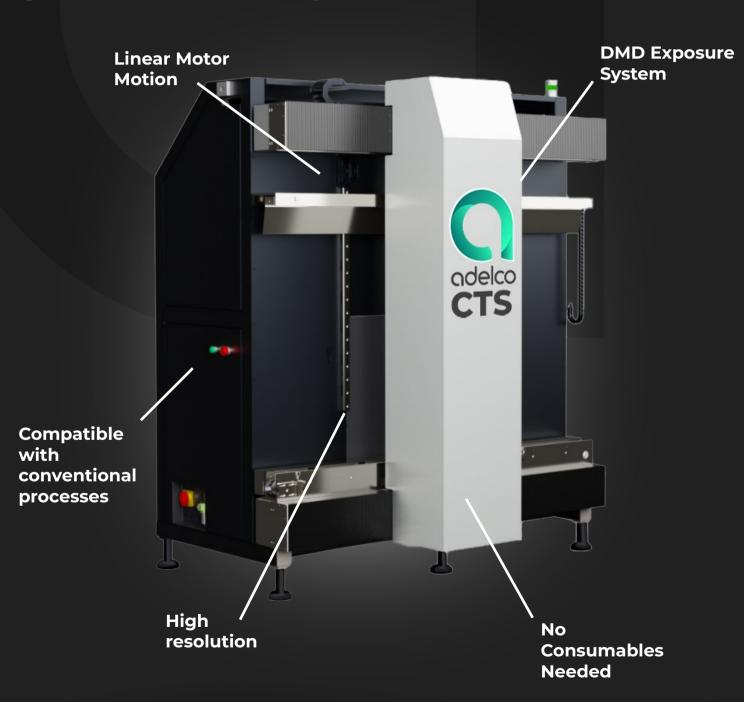
Adelco's **Laser V** system utilizes direct screen laser exposure technology to achieve **impeccable screen plate production.** It operates by directly reading data files through the computer to screen (CTS) system, converting them into images, and transmitting them onto screens using laser beams facilitated by the DMD and lens components.
