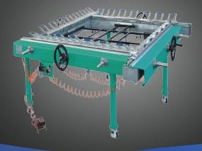
Our Adelco's Stretching equipment is suitable for screen printing screen high precision photographicc emulsion coating.
