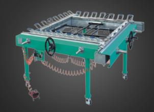
Adelco's stretching equipment is suitable for stretching screen printing screens. Easy to use, and incredibly precise. Suitable for stretching polyester, nylon and stainless steel material.
