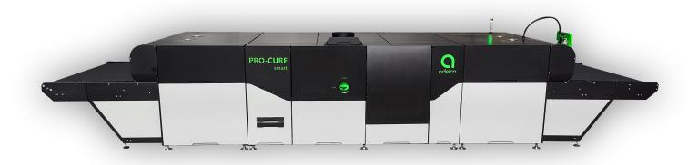
The new Adelco Pro-Cure Smart conveyor dryer range is available in four belt widths and five oven lengths, so you can customize your dryer to suit your individual curing requirements, for all digital and conventional textile ink systems. The Pro-Cure Smart is modular in design, making it the perfect option to add additional ovens to the dryer as your business grows.
