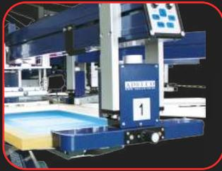
Three-way front and rear micro screen adjustment for easy set up.
