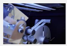
The LD70, is a new automatic machine developed for the placement of adhesive strips & labels for clothes. The purpose of the labels is to inform the final consumer about the size of the garment or other important information that the garment manufacturer deems appropriate.
