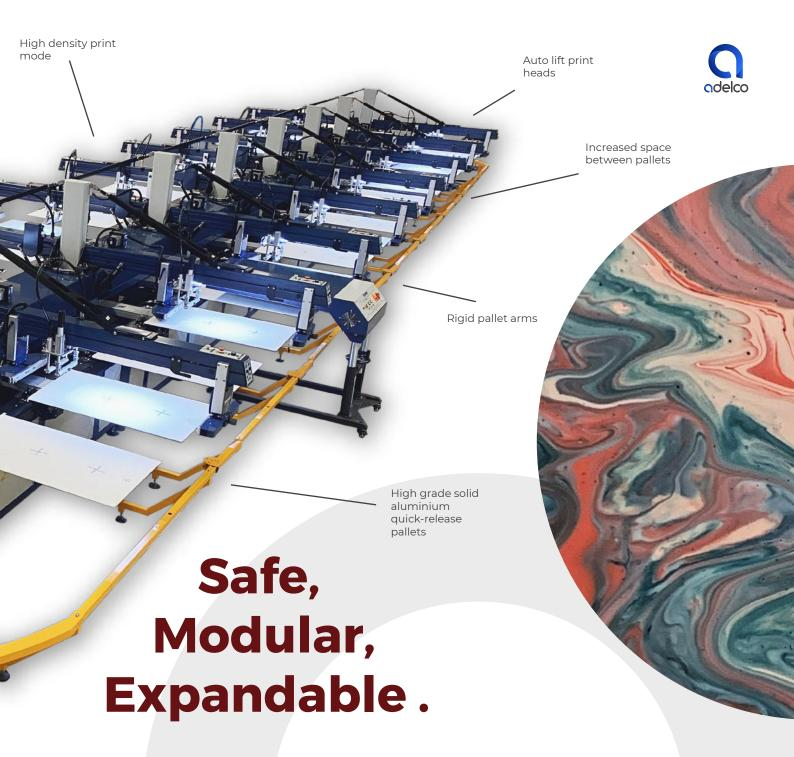
The Matrix Oval screen printing machine from Adelco offers a more efficient use of space thanks to its oval-shaped design. It offers greater stability with larger print press areas than comparable carousel based machines. The Matrix Oval provides more versatility with multiple flashes, cooling and specialty print stations, providing the most demanding ecological print solution.
