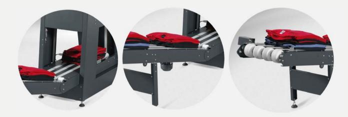
**NT50\*** is an automatic stacking machine, which can stack the already folded garments as they come from the **STP1000** automatic folding machine.
