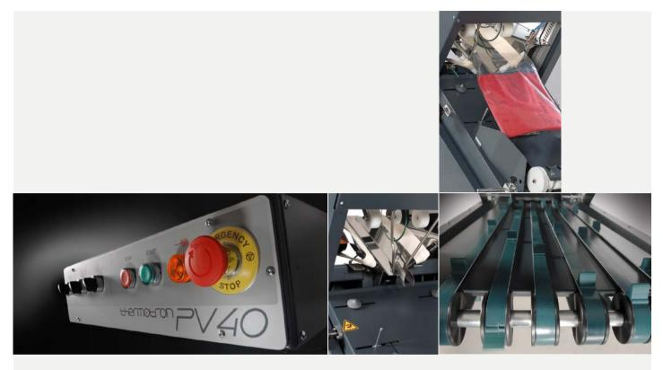
**PV40**\* is the new automatic bagging machine for garments and constitutes an evolution of its predecessor **PV38**, with targeted improvements and with a detachable transport belt according to the customer's needs. The output capacity of **PV40** depends on the output speed of **STP1000** or on how fast the operator places the garments in the machine when the machine functions independently.
