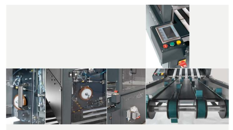
**KL60**\* is an automatic sealing machine that closes the bags that contain garments coming folded and packaged from the automatic folding machine **STP1000** and the bagging machine **PV40** with adhesive tape.
