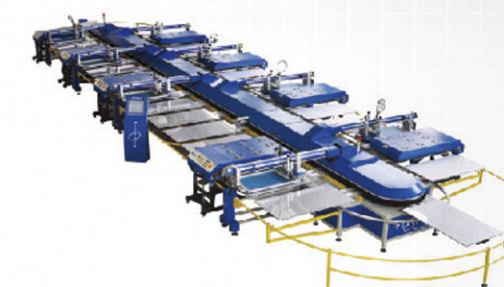
Model No: OPP-8C36S-80120 • 8 color 36 station • 80*120cm printing area
