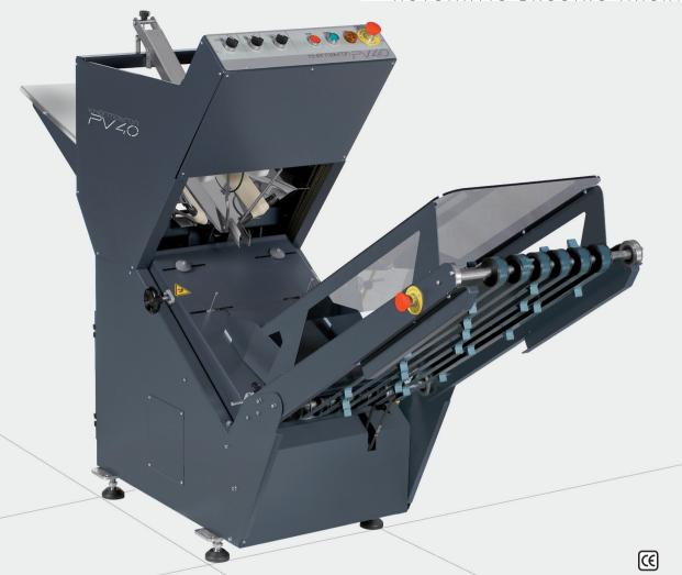
**PV40**\* is the new automatic bagging machine for garments and constitutes an evolution of its predecessor **PV38**, with targeted improvements and with a detachable transport belt according to the customer's needs. The output capacity of **PV40** depends on the output speed of **STP1000** or on how fast the operator places the garments in the machine when the machine functions independently.
